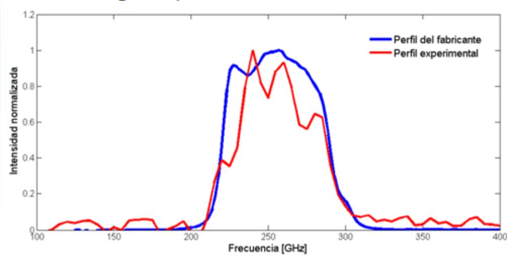
Millimeter (1.2mm) wavelength metal-mesh band-pass filter spectral profile measured in our lab.
