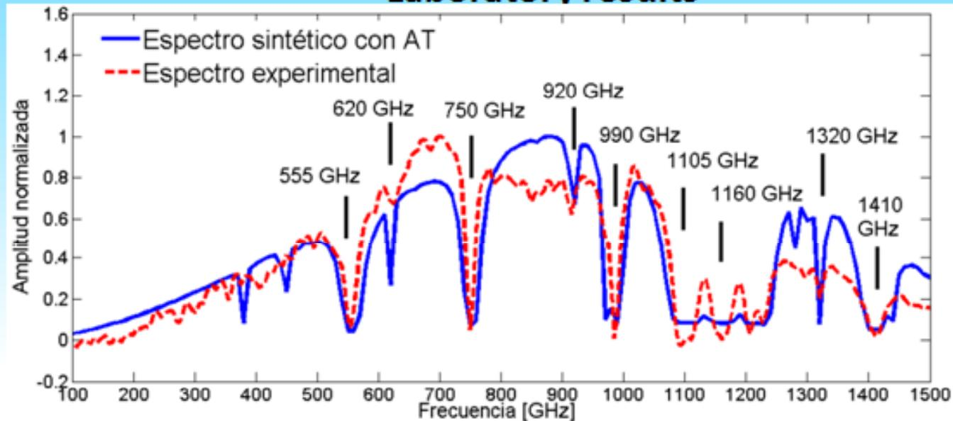
Atmospheric spectral profile of the atmosphere inside the FTS container measured in our laboratory which shows main water absorption lines and the range of operation of the instrument.
