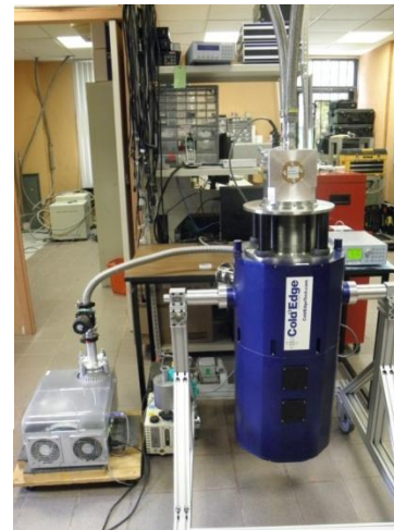
4-He Cryo-cooler, with a current closed cycle (from 4 K to 300 K). Nearly future from (0.3 K to 300 K). At the INAOE's facilities.
