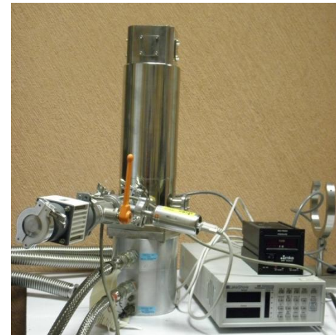
4-He Cryostat, with a closed cycle (from 10 K to 300 K), at the INAOE's facilities.
